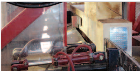
A single-block bridge timber being processed through a Mallotte gainer. Timbers are manufactured to exacting standards, numbered and packaged, and shipped to the end-use site for assembly.
