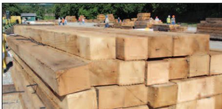
16-foot oak switch ties—end trimmed, incised, inspected, and ready to be trammed and treated.
