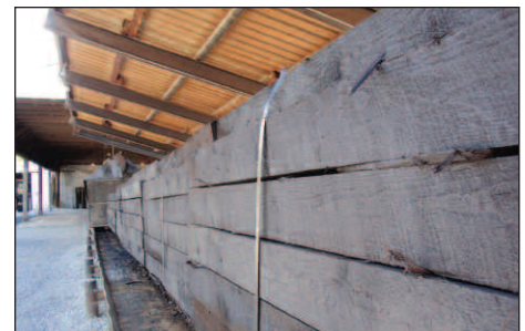
Acme Wood Preserving Inc. treats about 75-80 percent creosote wood ties (shown here), the balance CCA fence posts.
